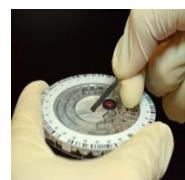
5. Remove the aluminum foil strip covering the sample injection port.
