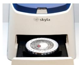
2. Hold a reagent disc by its edge. Gently place the disc into the drawer.
