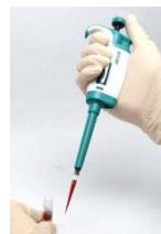
1. Use the provided pipette and tip to draw up 200 µL of the sample.
