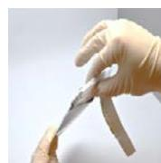
2. Grip with finger and thumb along with tissue paper to remove the reagent disc.
