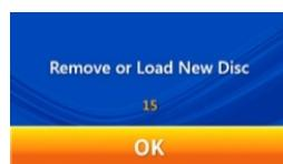
2. Press **HOME** to open the drawer and remove the reagent disc. An analysis is now completed.
