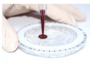
2. Keep the pipette **perpendicular** to the surface of the reagent disc. Gently push down the plunger to the lowest to dispense all the sample.
